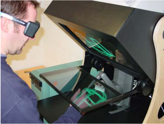
Figure 1: Phantom based 3D-Sketching system
