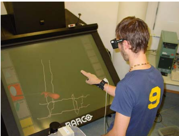
Figure 2: Gesture based 3D-Sketching system
