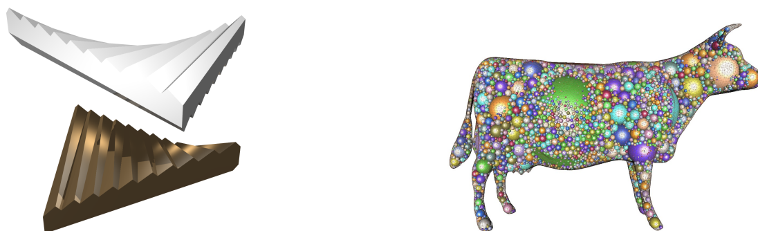
Figure 1: Left: the intersection of two Chazelle polyhedra is a worst case for polygon-based collision detection algorithms. It has a quadratic complexity. Right: our algorithm is based on space-filling, polydisperse sphere packings for arbitrary objects and, thus, independent of the object's surface complexity.
