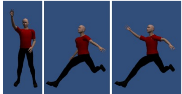
Figure 5: Initial reaching posture (left), initial jumping posture (middle), and reconstructed final posture (right) based on centre of mass (CoM) and inverse kinematic (IK) calculations.
