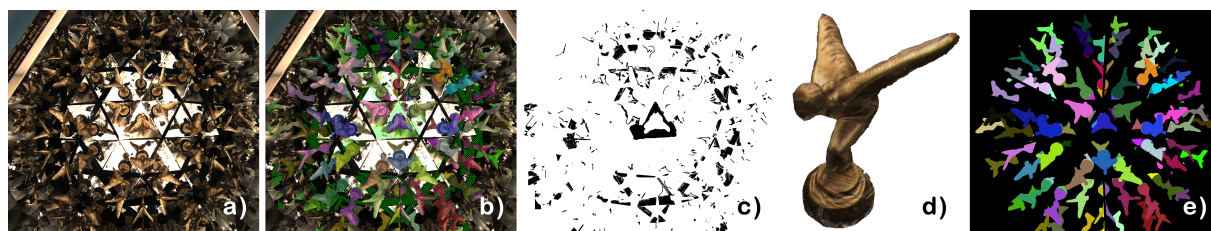
Figure 1: a) Input: Kaleidoscope image. b) User-drawn mask (green checkerboard pattern). c) User-drawn mask isolated. d) Approximate visual hull generated from (c) using image-based shading. e) Resulting labeling via visual hull.
