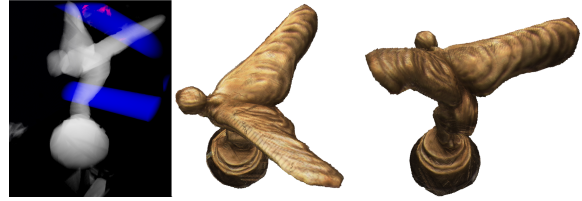
Figure 4: Semi-transparent mode (left): Depending on its state, each voxel is assigned color and density: part of the visual hull (white, low density), covered by the brush (blue, medium density), intersection of both (red, high density; top part of image). Image-based shading (middle and right): Color values are transferred from the kaleidoscope image.
