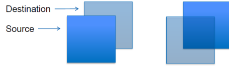
Left: Front fragment has higher screen contribution than the fragment behind and thus the color behind is rejected entirely. Right: Front fragment has lower screen contribution. It is rendered transparently.
