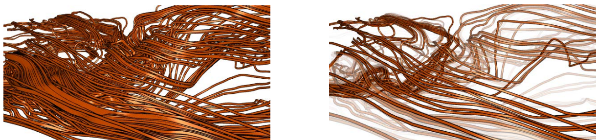
Figure 10: The random seeding on the left produces occlusion which makes it impossible to see the stream behind. Our approach (on the right) does not only improve the perceptibility. It can make structures visible that would be occluded.
