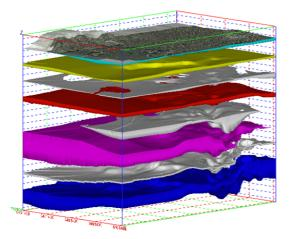
**Figure 1:** Stratigraphic units (exploded view) near a costal area in the western U.S. An aerial photo of the region is shown on the top layer. The color structures are aquifers and the silver structures are aquitards.
