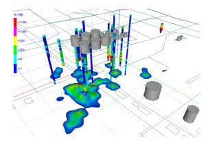
**Figure 3:** *LNAPL plume (color blobs), LIF responses (tubes of color spheres), and former aboveground storage tanks (ASTs) at a former gas plant in the southwestern U.S.*
