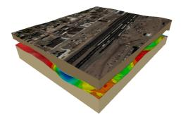
Figure 5: A two-unit structural model for a railroad site in the northern Midwest of the U.S. An aerial photo of the site was shown on the upper surface; the contact between the two units was illustrated as a series of colored iso-elevation contours.
