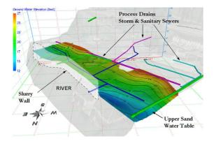
**Figure 2:** Potentiometric condition in an upper sand unit at a petroleum fuel terminal in the northwestern U.S. The transparent surface is the upland topography and river bathymetry.
