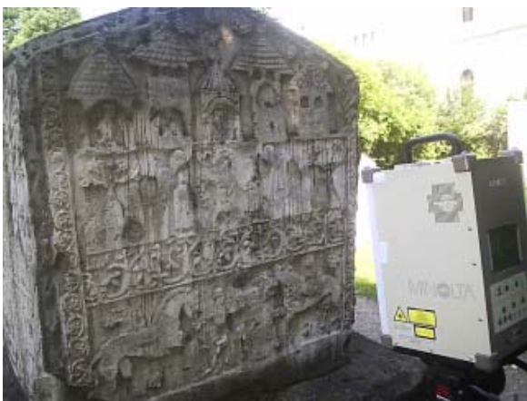
Figure 2. Minolta 910 laser scanner is a scanner for close range and indoor applications and has an accuracy of less than a millimeter.
