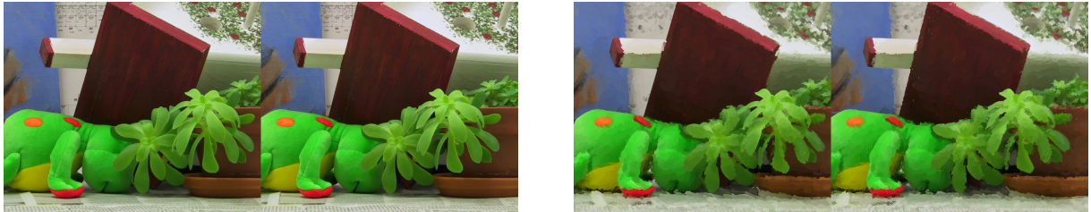
Figure 11: On the left, source image pair from Middlebury College, with provided ground truth disparity map. On the right, stereo pair generated by our algorithm.
