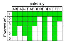
**Figure 6:** Work distribution on one GPU. Each column corresponds to a pair of objects, each row corresponds to a vertex of the first object of the pair. Filled squares are ray cast from the i<sup>th</sup> vertex of x, white square are padding as each object may have a different number of vertices.
