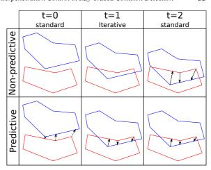
**Figure 3:** Comparison of predictive and non-predictive collision detection, with predictive rays the collision is detected earlier resulting in less interpenetration.
