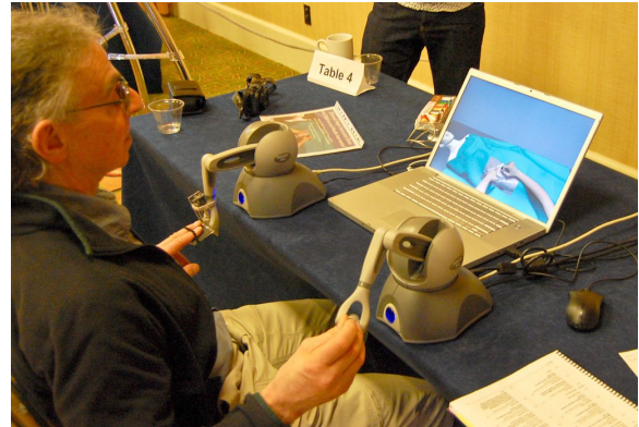
Figure 6: Mobile platform of the bimanual haptic simulator presented with the same haptic devices as in the stationary platform.
