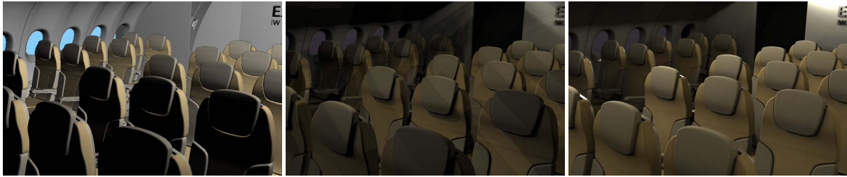
Figure 3: Screenshots showing the aircraft cabin scene (a) in the rasterization back-end, (b) in the ray tracing back-end directly after the switch from rasterization, starting the accumulation, and (c) with global illumination after 15 seconds of convergence.
