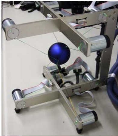
Figure 1: The haptic interface “SPIDAR”
