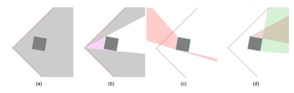
**Figure 3:** (a) A beam is created and intersected with the geometry. (b) The beam is split into child-beams, according to the intersections. (c) Reflection edges are identified, and the old beam origin is reflected at those edges, constructing reflected beams. (d) In the same manner diffraction beams are generated at silhouette edges.
