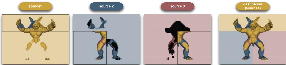
**Figure 1:** Sort-last rendering with direct send compositing using three channels. The first three images show the rendering buffers which contain the rendering of the partial database and the composited tile of this channel. The last image shows the final, visible destination view with the fully composited image. The channels use different clear colors to identify the tile layout.
