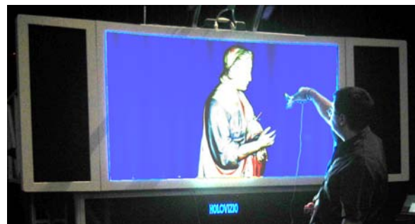
Figure 1: Massive model visualization on a 50Mpixel spatial 3D display. The display has a screen dimension of 1.6x0.9 meters, and provides continuous horizontal parallax. Interactive rates in the manipulation of massive geometric models are guaranteed by a cluster-parallel spatial 3D display aware coarse grained multiresolution technique.
