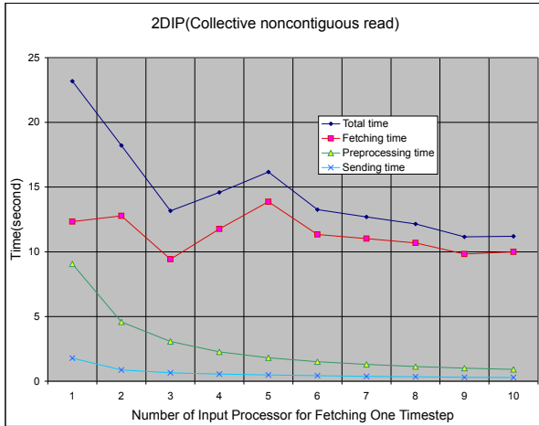
Figure 9: Using 2DIP strategy with Collective Noncontiguous Read, sending time is reduced to under 1 second which makes interactive visualization possible.
