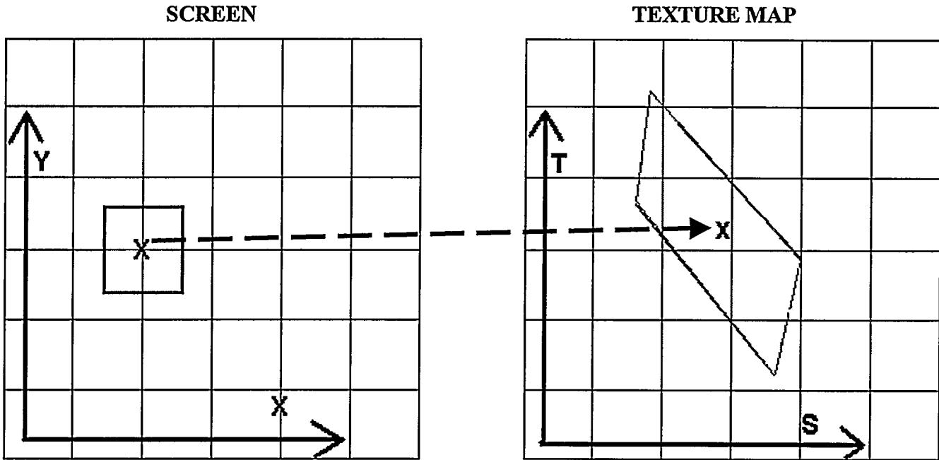
**Figure 5: The Projection of a Screen Pixel into the Texture Map**
