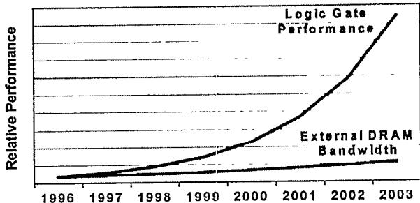
**Figure 1: On chip vs. External Bandwidth**
