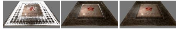
Figure 8: Quadtree relief mapping using a 512 \times 512 height map. White means not found within 10, 15 and 25 iterations.
