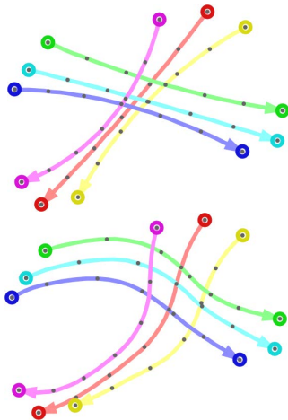
Figure 7: The first SAMBA pass (top) shows a collision between the two clusters. We show the result after 1000 SAMBA passes (bottom).
