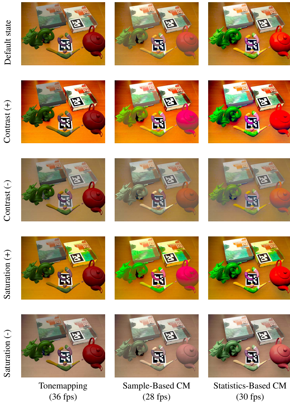
Figure 4.16: These images show a comparison between the tone-mapping operator of Reinhard et al. [113], the sample-based color mapping approach, and the statistics-based color mapping approach. Five different input images for the see-through camera were used with normal settings (first row), increased contrast (second row), decreased contrast (third row), increased saturation (fourth row), and decreased saturation (last row) created using a graphics editing program based on the image from the first row. The book on the right side and the table including the two BCH markers, are real objects while all others are virtual ones.
