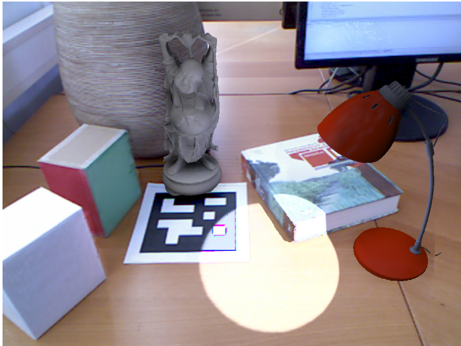
Figure 5.1: This figure shows a mixed reality scenario where a virtual table lamp illuminates the real and virtual objects causing indirect shadows on the real vase from the Buddha. The scene is reconstructed during run-time and rendered at 17.5 fps.
