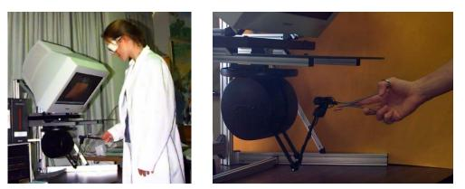
Figure 2-3 Mounting the PHANTOM Premium upside-down for increased range of motion in suturing procedure. Image courtesy of R. Webster.
