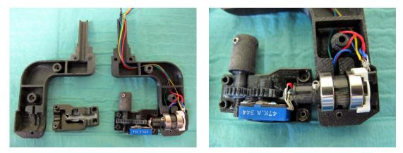
Figure 6-12 Left: Two halves of the modified wrist for the Omni force feedback device. Right: A close up image showing mechanics of the final two degrees of freedom. On the right of the image two sealed deep groove ball bearings can be seen on the end of which the Omni's original potentiometer is mounted. On the left of the image the blue off the shelf Tyco potentiometer can be seen, rotated via the dual cog assembly.
