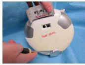
8.The silver dust protectors can be unclipped with a screwdriver
