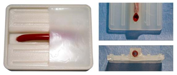
Figure 5-10 Left: The left hand side of the tactile end effectors silicone has been removed to reveal the simulated femoral artery. Right: The profile of the tactile end effector can be seen in the removed silicone section. A simulated femoral artery has been inserted to illustrate its path through the silicone. The ridged profile of the silicone secures it to the plastic base during use.
