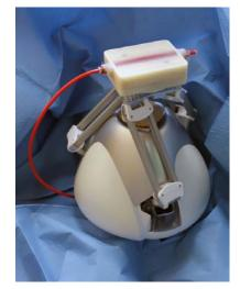
Figure 6-1 Modified Novint Falcon force feedback device. The Falcon has been rotated through 90 degrees and mounted with the first prototype of the hydraulically actuated tactile end effector.
