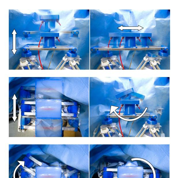
Figure 6-7 Multiple images are overlaid on top of each other to demonstrate the dual Novint Falcon's Five force DOF and the tactile end effector's one degree of freedom. Multiple images of the devices range of movement have been superimposed to demonstrate the possible range of motion. The device offers three force DOF translation and two torque DOF. A single redundant DOF is produced by a servo housed within the tactile end effector (bottom left).
