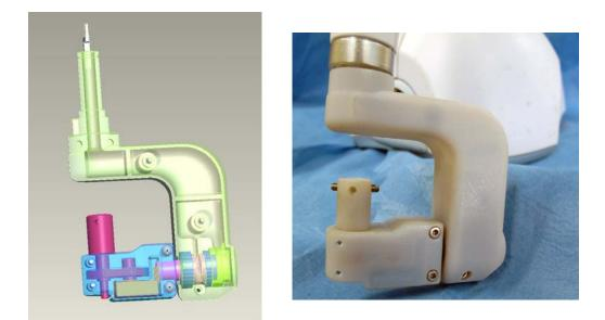
Figure 6-11 Left: A Pro Engineer model of the redesigned Omni wrist. Right: The manufactured wrist structure fitted to an Omni device.
