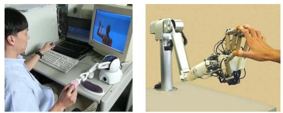
Figure 2-13 Left: A brachial pulse palpation simulation [74] Right: Haptic Interface Robot (HIRO) [75]
