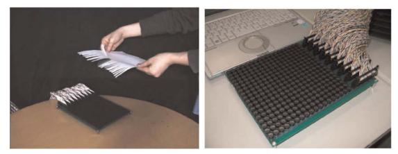
Figure 2-4 A non-contact tactile display based on the radiation pressure of airborne ultrasound provides haptic feedback through air [20].
