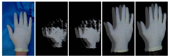
Figure 4-4 The acquisition stage, From Left to Right: A faint red selection target can be seen in the video image of a users hand ta<sup>nd</sup>: The hand extracted after a single chrominance acquisition pass. 3<sup>rd</sup>: Two acquisition passes. 4<sup>th</sup>: 10 acquisition passes. 5<sup>th</sup>: 20 acquisition passes.
