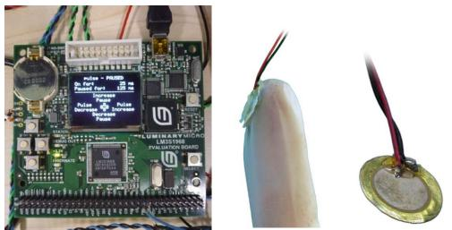
Figure 5-3 Left: An integrated circuit board Luminary Micro used to control the pulse displacements of the piezoelectric and micro speaker hardware. Centre: A piezoelectric pad fitted to a surgical glove. Right: A piezoelectric pad removed from its audio housing.
