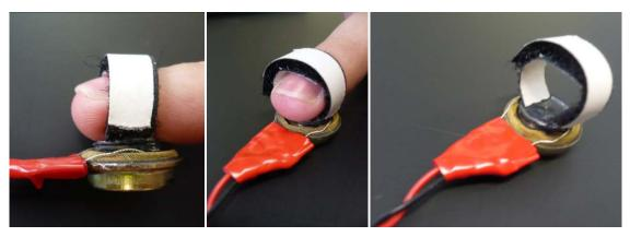
Figure 5-5 Finger mounted micro speaker tactile device.
