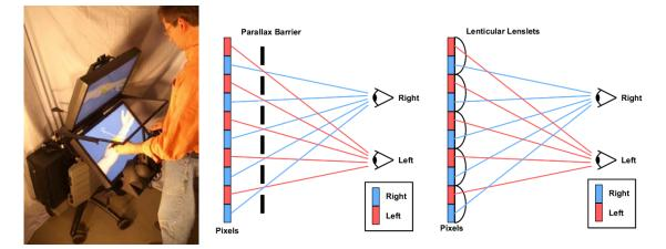
Figure 2-9 Left: Haptic interaction using a Planar display (Picture courtesy of SimQuest). Centre / Right: Methods of passive autostereoscopic display. Images from www.3d-forums.com, last accessed o6/11/2010.
