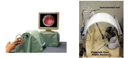
Figure 2-24 Left: HystSim from VirtaMed. Right: Laparoscopic adjustable gastric band simulator hardware [41]
