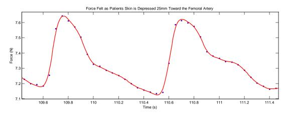
Figure 5-2 A 2 second sample of *in vivo* pulse force measurements at skin displacement toward the femoral artery of 25mm, an average applied force of 7.265N (over a complete measurement) and an average pulse fluctuation of 0.483N
