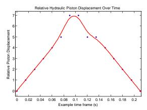
Figure 5-8 An example of the piston displacement used to produce a realistic pulsing sensation at the tactile end effector.
