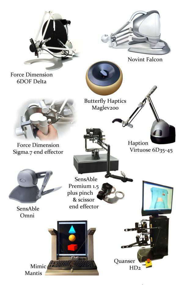
Figure 2-5 Commercial Force Feedback Hardware. 1<sup>st</sup> line – Manufacturer, 2<sup>nd</sup> line - Device Name
