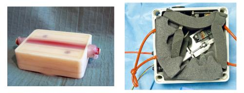
Figure 5-9 Left: First tactile prototype with rotating base. Right: The sound insulated servo driven hydraulic actuation unit. The device is hung underneath the force feedback hardware to eliminate audible vibrations.
