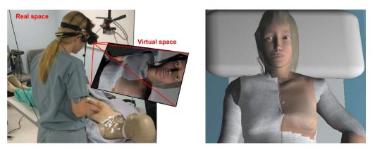
Figure 2-15 A breast palpation simulation using passive haptics and a HMD visualization [83].
