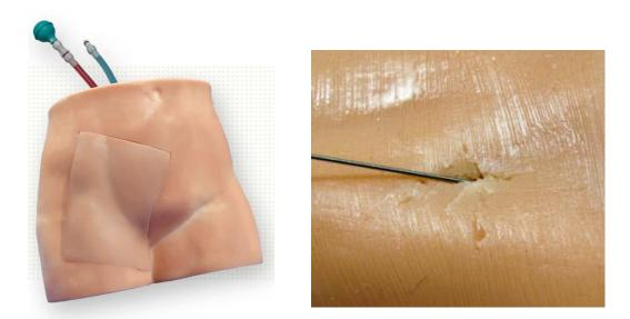
Figure 3-5 Multiple needle and wire punctures can cause rapid degradation of mannequin models. Left: FemoraLineMan from SimuLab (Seattle, USA). Right: puncture of CentralLineMan, SimuLab.
