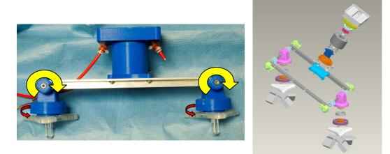
Figure 6-6 A modified end effector connects two Falcon devices to produce a custom 5 force DOF device. Two sets of dual revolute joints are used (one yellow rotation and one red rotation), connected to each Falcon via the clear plastic interfaces. The silicone tray tactile interface is mounted in the centre of the connecting bar.
