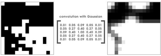
Figure 4-5 Passing a 5x5 Gaussian filter over a 15x15 subset of dataset C. Left image depicts a first incomplete capture of the hands chromatic range. Elements of value zero are rendered black, those of value 255 (hand) white. By applying a Gaussian filter to the data, neighbours that are not discovered to be hand but are surrounded hand coloured pixels will also become hand. Pixels at the boundary, will acquire a value between 0 and 255 and will be rendered semi opaque.
