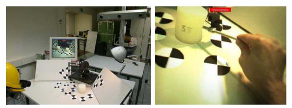
Figure 2-32 HMD augmented reality. Left: The major components of the system (Optotrak in background, the PHANTOM, the lamp, the landmarks placed on three different planes to cover the user's field of view involved in the system) Right: The stylus interface used to manipulate virtual objects. Images taken from [157].
