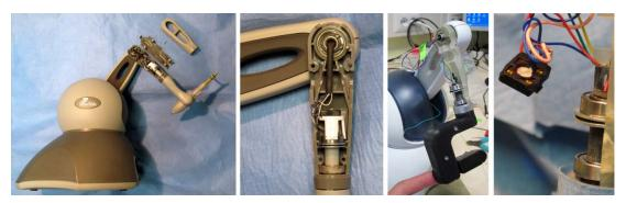
Figure 6-13 Left: The Omni's cover can be detached by removing a single screw on the arms underside. Four screws then need to be removed to uncover the internals of the arm, seen  $2^{nd}$  from left. After sliding the arm out, the new arm can be inserted,  $2^{nd}$  from right. Right: The Omni's potentiometers must be re-connected to the correct wires.
