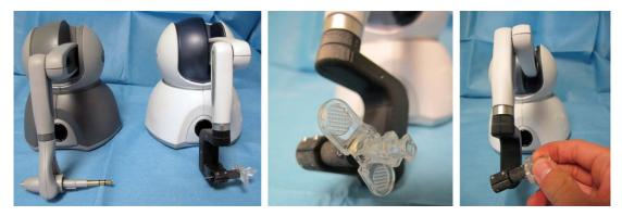
Figure 6-14 Left: A visual comparison of the off the shelf Omni with stylus removed and modified end effector. Centre: The needle hub mounted within the Omni end effector, providing high fidelity visual and tactile feedback as grasped. Right: The modified Omni as gripped by a user.
