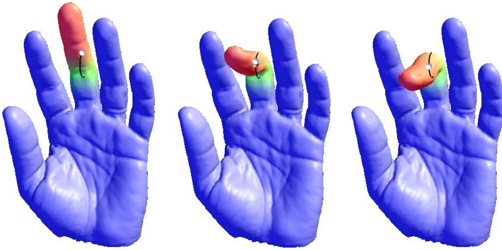
Figure 4.6: Using the geodesic distance field of a point on the tip of the middle finger, we can deform the finger without affecting other parts of the shape.
