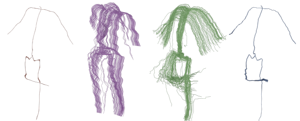
Figure 5: Qualitative comparison of each model's invariance to reparameterization. We display 100 resampled versions of a single shape graph (orange) and the 100 reconstructions produced by PointNet (purple), DGCNN (green), and VariGrad (blue).
