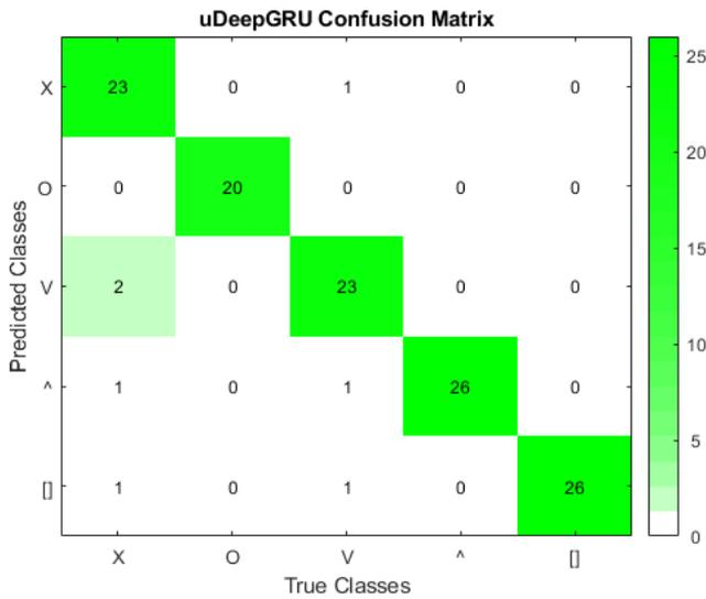
Figure 6: Confusion matrix of the uDeepGRU<sub>2</sub> run, considering only the classification attempts in the correct time window.
