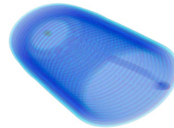
Figure 4: Geometry at a low resolution can be described by a fuzzy point cloud; i.e. a point cloud in which each point is normally distributed in space. This illustration shows such a fuzzy point cloud. Each point is drawn as a semi-transparent sphere whose radius corresponds to a fixed probability – an isosurface in probability space.
