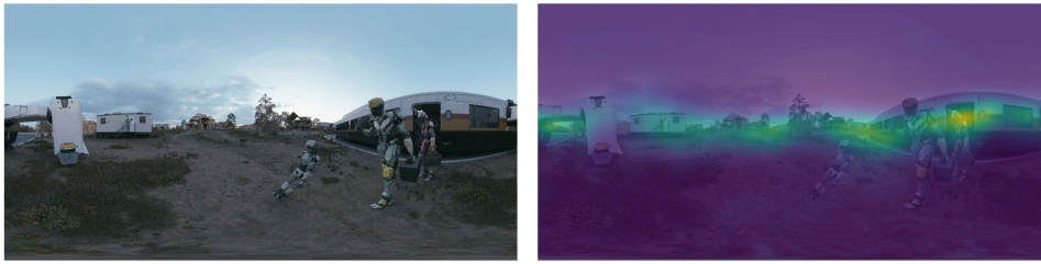
Figure 4.5: Saliency maps show the likelihood of users directing their attention to each part of the scene. Most of the current literature has been devoted to estimating saliency in unimodal, visual stimuli. This image shows the recent visual saliency estimation method proposed by Martin et al. [220] ( Left : Input panorama. Right : Estimated saliency). It has been shown that each sensory modality has the potential of influencing users' attentional behavior, therefore, there is a need for further exploration of multimodal saliency in VR.
