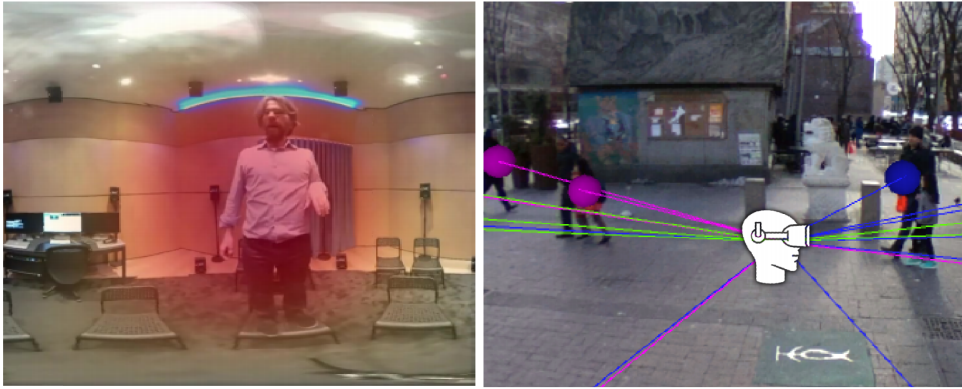
Figure 4.3: Including correct and coherent auditory information in the virtual environment has been proved to increase realism and immersion. Left : A system that automatically generates ambisonic information that creates a smoother acoustic experience for the scene [246]. Right : A framework to include auditory information into 360° panoramas depending on the elements in the scene [146]. In both cases, their validation experiments yield users' preference when auditory information is included, and an overall increase in the perceived realism and immersion.
