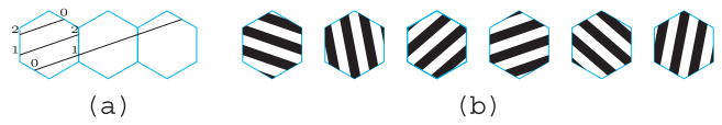
Figure 16: (a) Choosing a slanted line direction for decorating 6-way weave tiles. The line shown starts at a mid-point of one edge, and crosses 2 edges before reentering back in its starting position. (b) A working set of raw tiles developed observing similar considerations to the 4-way case (Figure 13).
