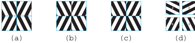
Figure 13: Developing 4-way weave tiles: (a) Two tiles which weave well along vertical edges, but there is no reasonable way to resolve priority along horizontal edges. (b) Which line goes above/beneath is clear here, but weaving is not symmetric on the sides of the horizontal edge between tiles, which would later make aligned edges appear offset. (c) Two tiles which weave perfectly along both horizontal and vertical edges, and (d) a working set of 4 tiles comprising the two in (c) and their 90° rotations.
