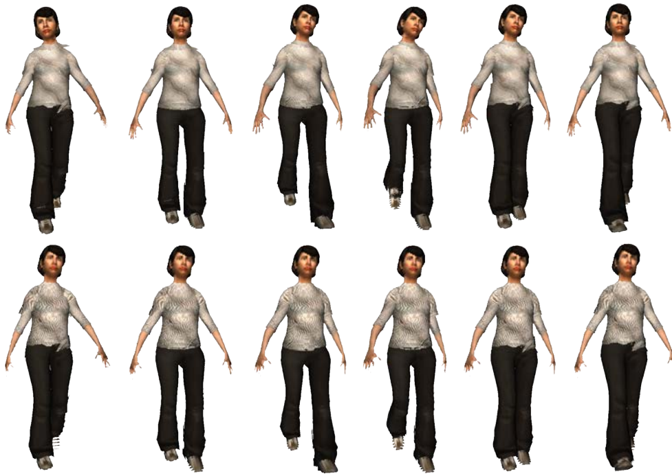
FIGURE 6.8: Rendering relief impostors with 21 bones (top) and 7 bones (bottom). Note that in the 7-bone representation the head bone has been collapsed with the trunk and thus both undergo the same transformation.
