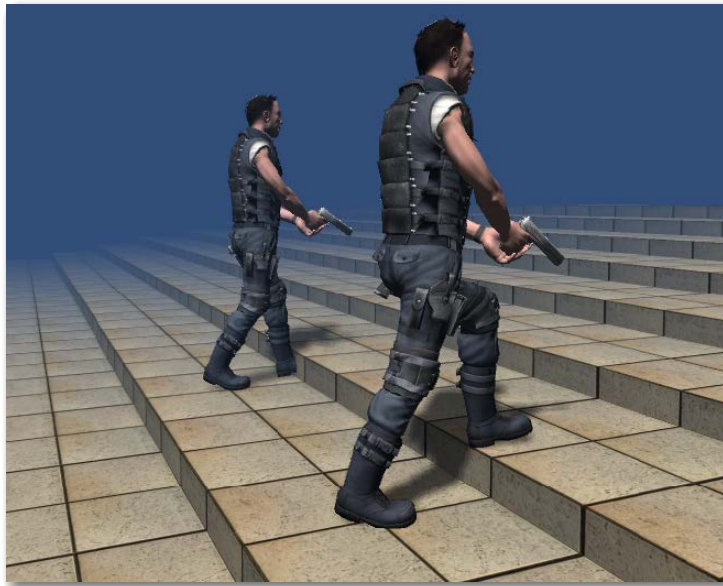
FIGURE 3.19: Comparison of synthesized motion of human character with semi-procedural adjustments (foreground) and without (background). [Johansen, 2009]
