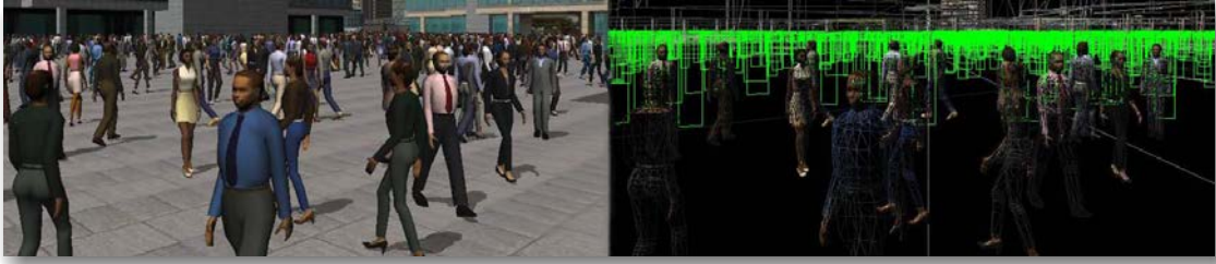
FIGURE 3.31: Geopostors. Far agents are rendered with impostors while closer ones are rendered with geometry. [Dobbyn et al., 2005]
