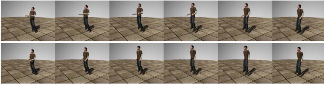
FIGURE 3.21: A user can fine tune an animation by incrementally adding constraints: (top) jumping generated by the user using five key trajectories (both hands, both feet, and root); (bottom) a slightly different jumping motion generated after adjusting the positions of the hands at the top of the jump. [Chai and Hodgins, 2007]
