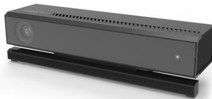
FIGURE 3.14: Microsoft Kinect 2.0 is a low cost depth camera. One of its applications can be to perform markless motion capture.
