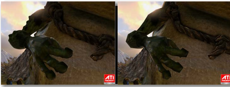
FIGURE 3.35: Tessellation allows rendering large crowds of characters with extreme details in close-up (left). The same character without using tessellation looks significantly less detailed (right). [Tatarchuk et al., 2008]
