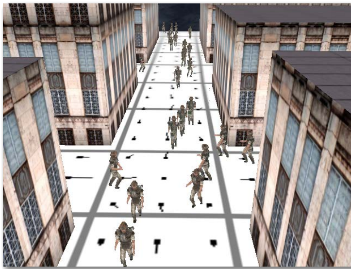
FIGURE 3.7: A frame showing people moving through a city, driven by a flow tiling of the streets. Internal boundary conditions prevent people from walking through building walls. [Chenney, 2004]
