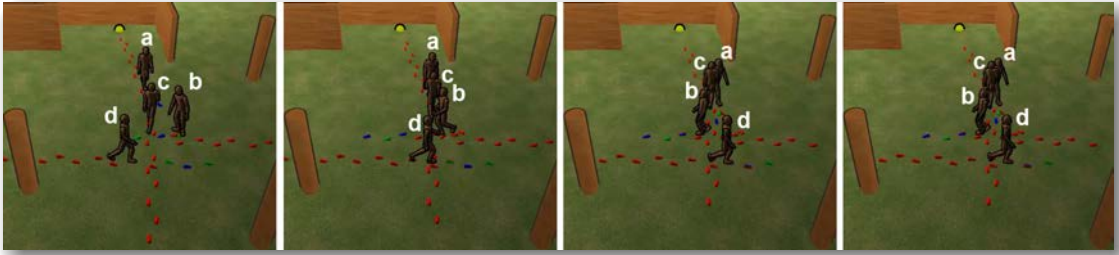
FIGURE 4.18: Example with four agents crossing paths with a drastically reduced search time resulting in agents a and c not being able to avoid intersection as seen in the last two images of this sequence. Also notice how agent b , walks straight towards c , steps back and then continues, instead of following a smooth curve around c .
