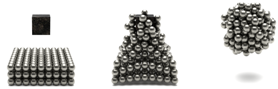
Figure 18: A cubic magnet stably attracts 243 small metal balls, simulated by integrating the BEM-based magnetostatic solver into Bullet Physics SDK [Cou15]. Source: Ni et al. [NWWC24].
