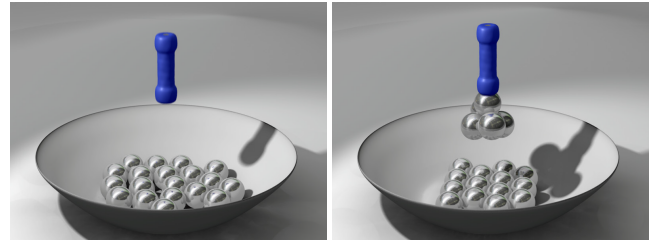
Figure 13: Snapshots of an interactive simulation in which soft ferromagnetic spheres are lifted by a permanent magnet. Source: Thomaszewski et al. [TGPS08].
