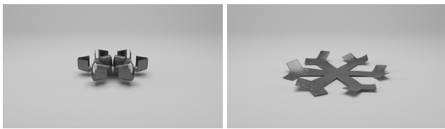
Figure 21: A deforming thin-shell hexagram, which is consistent with real-world experiments [KPLZ19]. Left: curling up; right: arm-shaking. The magnetization profile is optimized using the implicit FEM framework. Source: Chen et al. [CNZ*22].
