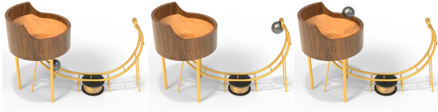
Figure 16: A magnetizable ball is running indefinitely from the funnel into the tracks and loops back into the funnel. The additional momentum for the ball to loop back into the funnel is provided by turning on and off an electromagnet at the correct time. Source: Westhofen et al. [WFJB24].
