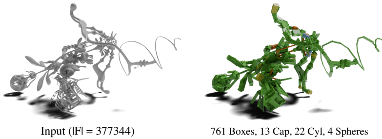
Figure 24: Our approach on a particularly challenging mesh, “Yeahright”. Our approach can preserve thin structures and holes. ©Keenan Crane.
