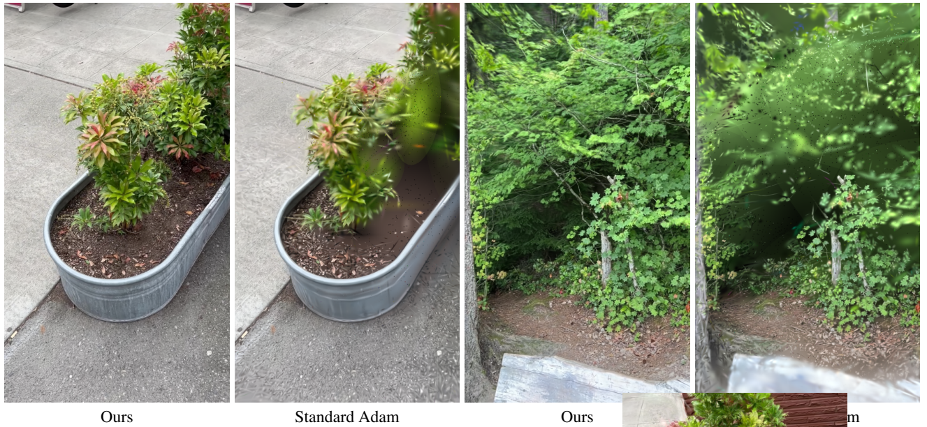
Figure 8: Standard Adam updates all parameters on every iteration irrespectively of whether the primitives are visible in the rendered image, leading to divergence, particularly in cases when the primitives are obscured, or when they have small area.
