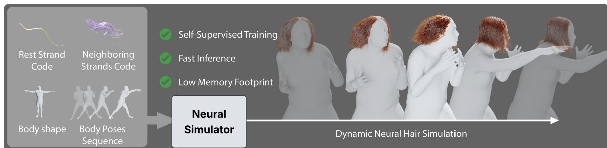
Figure 1: We present Neuralocks, a novel method that achieves high-performance dynamic neural hair simulation with a compact network size. This makes it a suitable solution for deployment on lower-end devices, which are commonly used in games and interactive experiences. At the core of Neuralocks lies its ability to generate strand-level deformations by leveraging boundary condition history and local lock neighborhood information, enabling realistic and detailed hair simulations. Our method is fully self-supervised, eliminating the labor intensive and expensive process of generating simulated training data.
