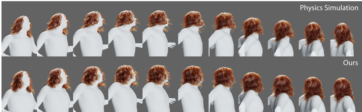
Figure 9: Physics Simulation Comparison We evaluate our neural simulation results against those of a widely adopted, highly efficient XPBD simulation model. While physics-based simulations offer the highest quality results with dynamic behavior, they come at a significant computational cost. In contrast, our neural method captures the dynamic behavior of hair, albeit with more damping, but achieves this at a fraction of the computational cost.
