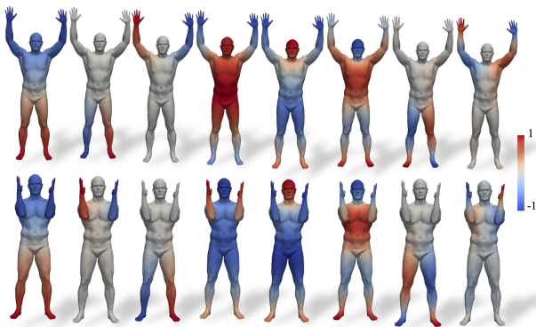
Figure 4: The first eight eigenvectors of the LBO on two near-isometric shapes. They are invariant up to a sign flip. Further, the eigenvectors corresponding to larger eigenvalues (right) oscillate more than the eigenvectors of smaller eigenvalues (left). Taken from [BRGK23].
