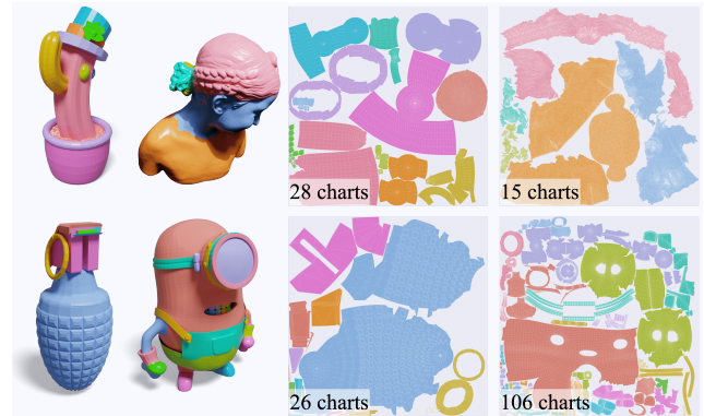
Figure 4: Mesh parameterization maps a 3D surface to a 2D domain (UV space) by partitioning it into charts and flattening each into a planar region. Example meshes (left) and UV layouts (right) show varying chart counts. Figure adapted from [WWS*25].
