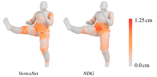
Figure 7: A comparison of VertexNet and NDG with respect to per-vertex accuracy. For each skin vertex, the average distance of both the skin vertex and its corresponding muscle vertex to their respective target position is visualized. NDG attains E_{\text{pos}} = 1.81 mm, while VertexNet attains E_{\text{pos}} = 2.27 mm.
