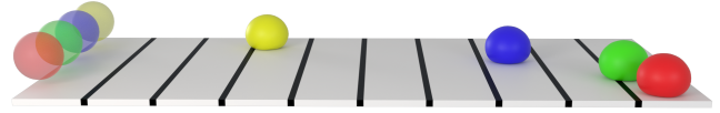
Figure 3: Rolling sphere. A deformable sphere with initial horizontal velocity rolls on a flat surface. Different Newton step velocity tolerance are used: 10^{-1} \text{ms}^{-1} (yellow), 10^{-2} \text{ms}^{-1} (blue), 10^{-3} \text{ms}^{-1} (green), 10^{-4} \text{ms}^{-1} (red).
