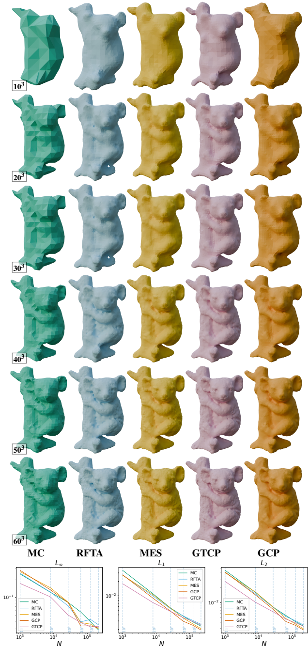
Figure 16: (top) Contouring results on regular grids of SDF samples of the KOALA model. (bottom) distance metrics to the ground truth mesh (log-log).
