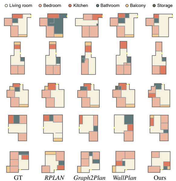
Figure 13: Comparison to the state-of-the-art techniques on the boundary-constrained generation. Each row shows the generated floorplans by different methods applied to the same architectural boundaries. We demonstrate the results of the ground truth, RPLAN [WFT*19], Graph2Plan [HHT*20], WallPlan [SWL*22], and our method, respectively.
