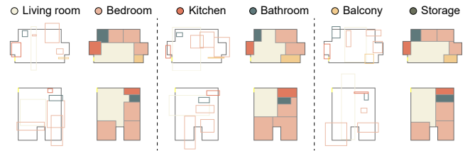
Figure 23: Extreme tests for geometry-semantics optimization. We apply significant perturbations to the ground-truth room layouts to obtain poor-quality initial room layouts.
