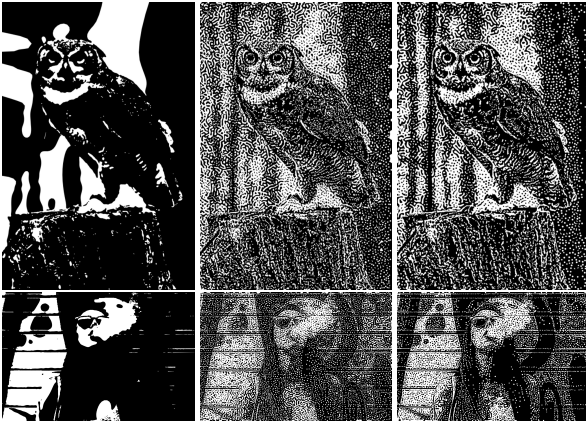
Figure 3: Effect of error diffusion and manipulation. Left to right: \alpha = 0 (no error diffusion); \alpha = 1 (regular error diffusion); dynamic alpha using our proposed method.
