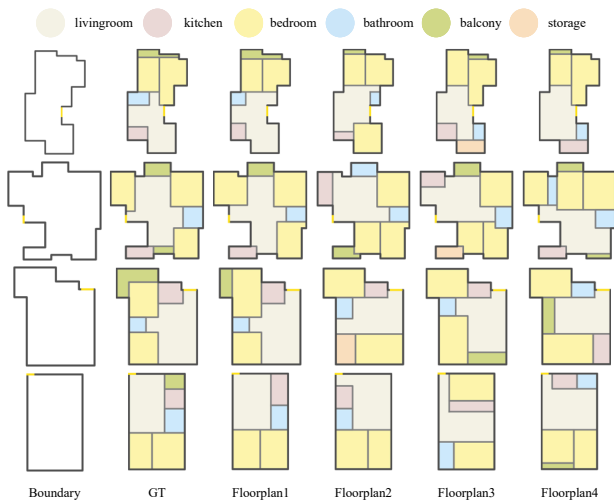
Figure 7: Diverse floorplans from a single boundary: our method generates multiple layouts for the same input boundary, demonstrating sampling variability and design flexibility.
