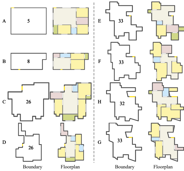
Figure 9: Generalization to extreme boundaries. The numbers denote boundary vertex counts, demonstrating robustness to complex shapes beyond the training distribution.
