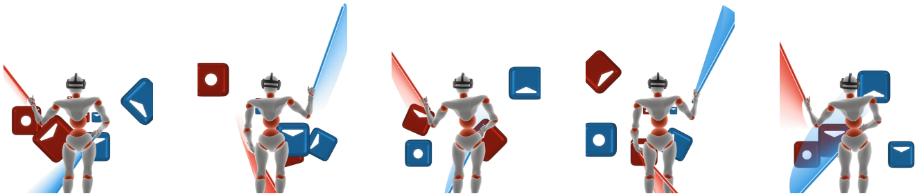
Figure 10: The physics-based version of Robo-Saber plays colored notes. The red and blue notes are correctly cut in sequence, with matching saber colors and directions. The dotted notes can be hit from any direction.
