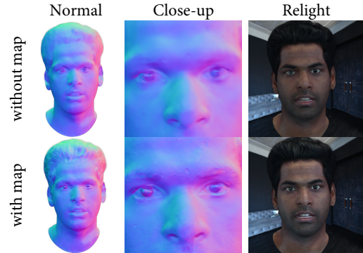
Figure 9: Ablation test on the normal map. 3D reconstruction is performed without relying on the normal map, i.e. normals are only computed from the Gaussian splats and fine surface details are baked in the other channels (top row), compared to reconstruction with a normal map (bottom row).
