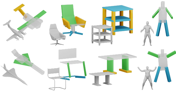
Figure 6: Using our cuboid abstraction to decompose shapes into its geometric parts enables us to perform partial symmetry detection. Colors indicate groups of symmetric parts.
