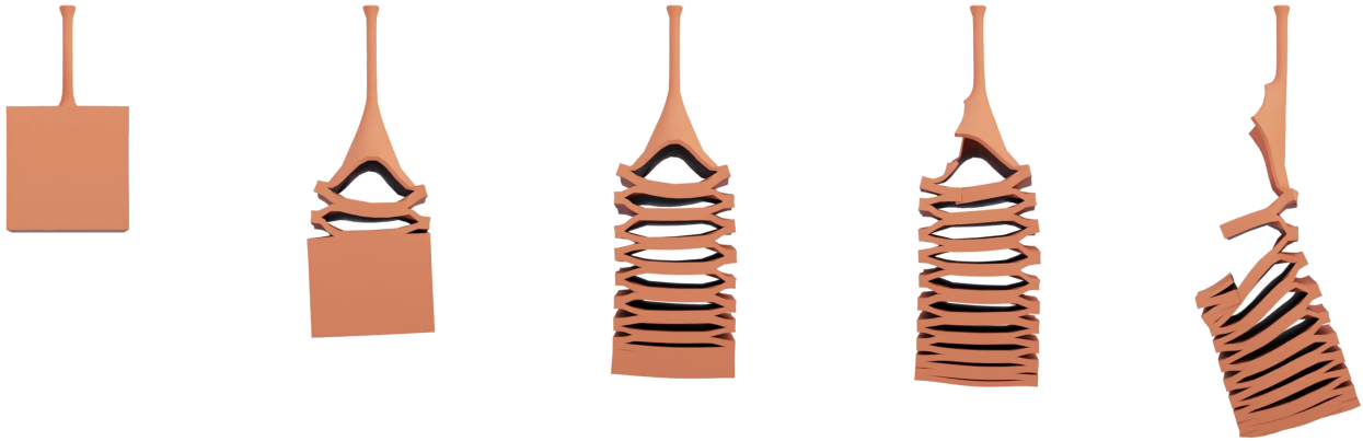
Figure 7: An elastic hanging cube is cut horizontally multiple times, resulting in an accordion structure. The last cut rips apart the top layers.
