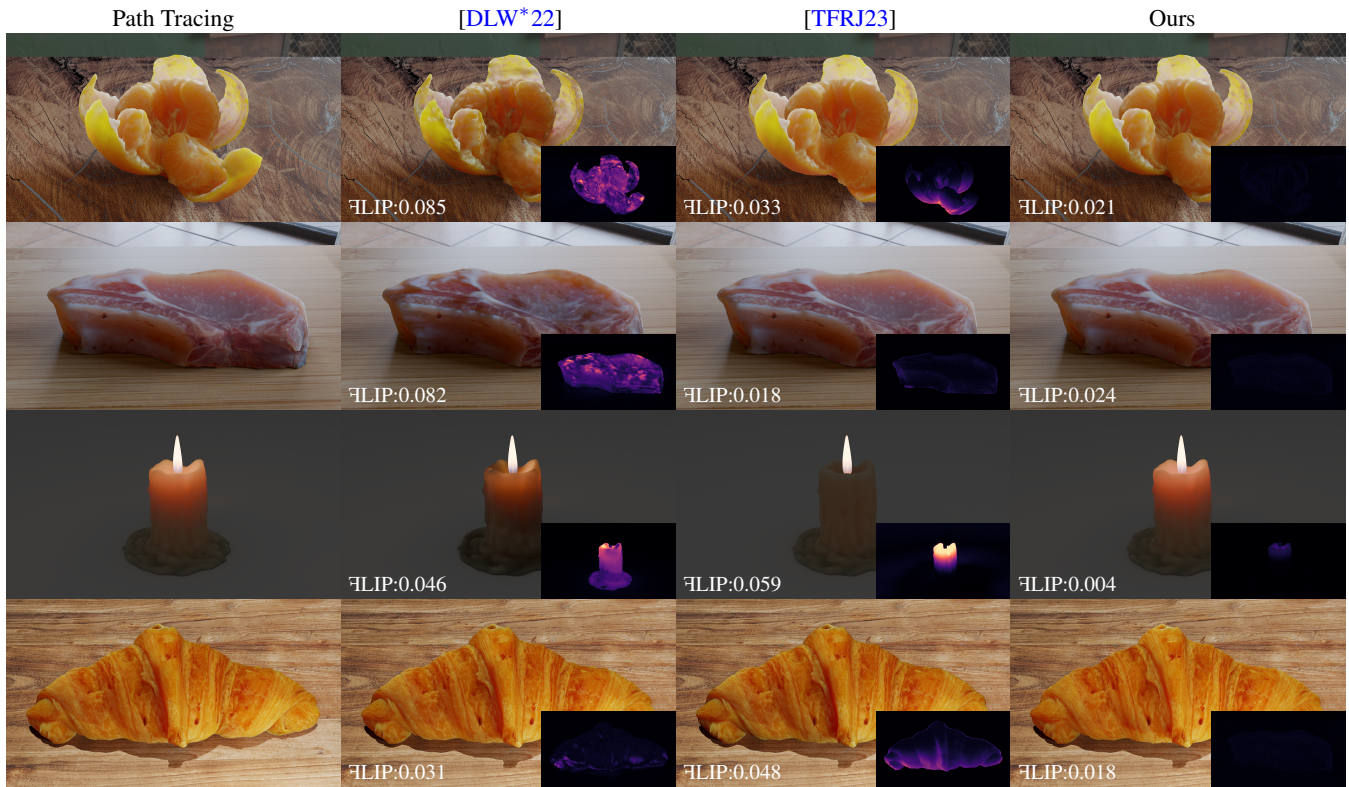
Figure 7: Comparison with reference path tracing and recent work on representing the appearance of a heterogeneous translucent object: Deng et al. [DLW*22] using textured parameters for the standard dipole model, which was derived for homogeneous half-space materials, and TG et al. [TFRJ23] using a neural representation limited to distant lighting. Our model most closely matches the path traced references (see the inserted FLIP mean and error maps). The FLIP error maps clearly highlight the limitations of the models we compare with.
