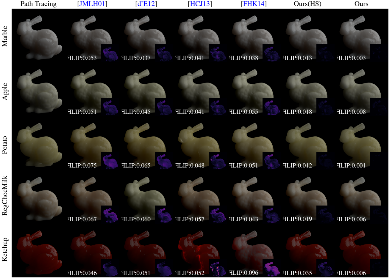
Figure 9: Comparing the half-space (HS) and the full geometry versions of our method to various diffusion based approximations. Path traced single scattering was added to the models not including single scattering [JMLH01, d'E12]. At the bottom of the images, we include per pixel and mean FLIP scores (lower is better) with respect to the reference path traced images. The half-space (HS) version of our model produces quality consistently better than the diffusion-based models, while the full geometry version matches the reference very well. The optical properties for the materials are marble, apple, potato, and ketchup [JMLH01] as well as regular chocolate milk [NGD*06].
