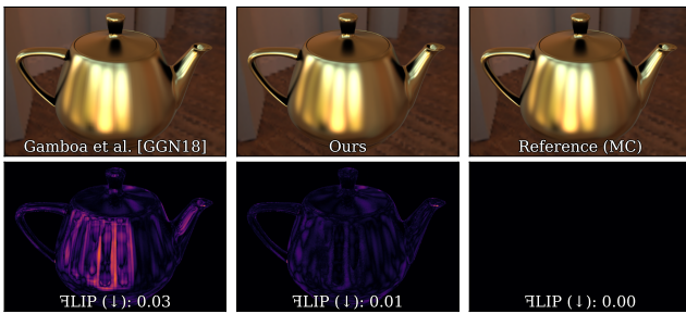
Figure 7: Comparison between precomputed [GGN18] and our on-the-fly computation of NDF_{SH} coefficients. The (2\times) FLIP difference (bottom row) shows that our method eliminates block-like artifacts stemming from the discretization of stored SH coefficients.
