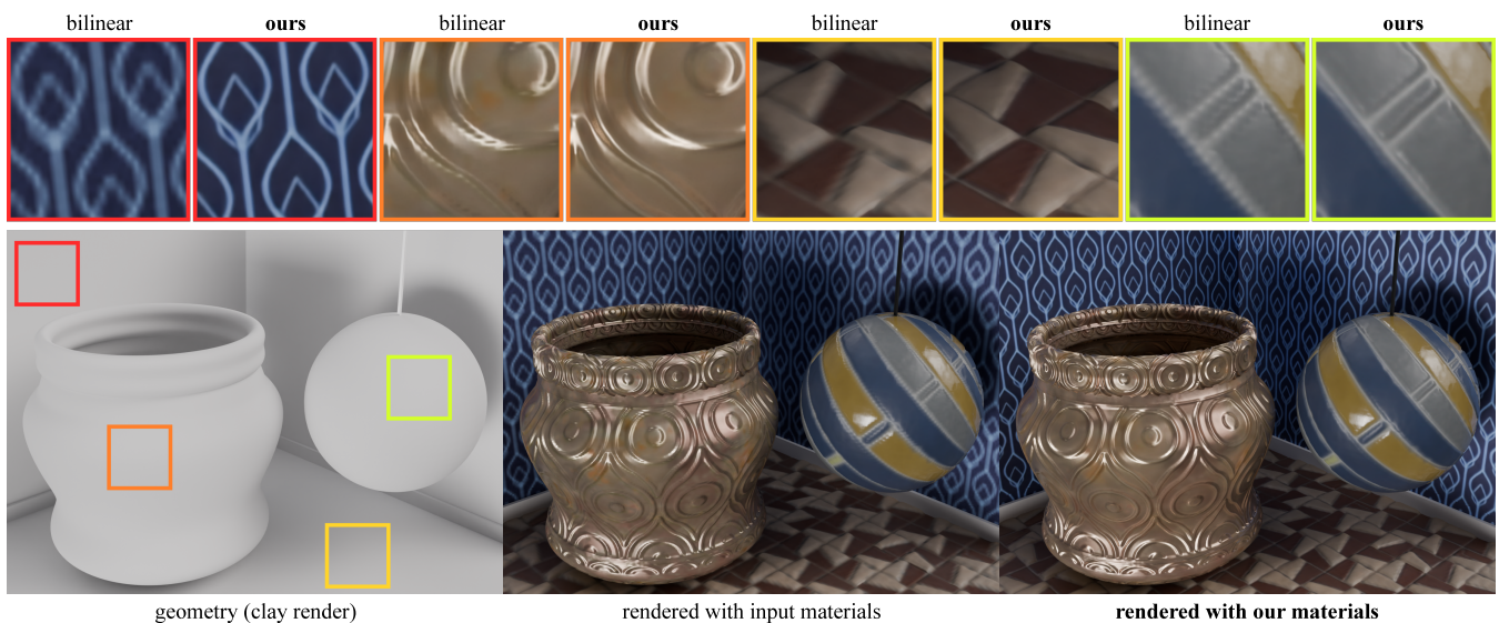
Figure 1: Given a low-resolution 128^2 input materials, our method produces 512^2 outputs preserving tileability and displaying sharper material structures compared to widely-used per-channel upsampling filters (e.g. bilinear or Lanczos) in less than a minute.
