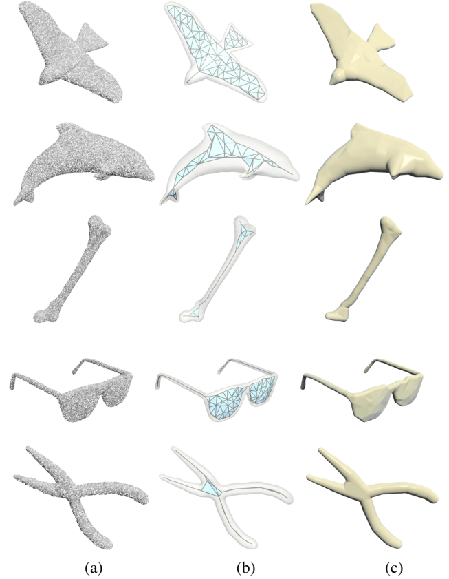
Figure 11: Shape skeletonization results for triangle soup. (a) Input triangle soup. (b) Skeletonization result. (c) Shape reconstruction.
