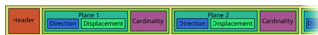
Figure 11: Output bitstream. The header describes the root cell and total cardinality. Each section provides three elements: the bisecting plane direction and its displacement, and the cardinality.
