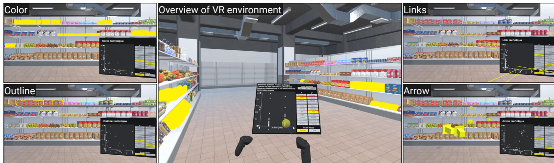
Figure 1: In our user study, we present a virtual supermarket with four highlighting techniques. Center: First-person view of the supermarket while brushing a scatterplot, with products on the shelves highlighted. Top left: The Color technique. Bottom left: The Outline technique. Top right: The Link technique with products behind the camera selected. Bottom right: Still image of the Arrow technique.
